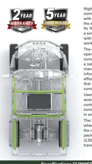
High powered performance you can count on. The GREENWORKS<sup>®</sup> commercial utility vehicle (UTV) is designed to go the distance with its powerful 16kW max gTRON<sup>™</sup> drive system, operating with the equivalent power of a 31hp / 496cc displacement petrol engine. Its 16kWh battery module provides up to an impressive 120km on a single charge for all day use. This vehicle is up for any challenge with superior off-road performance and on-demand 4WD for a true work utility experience.
