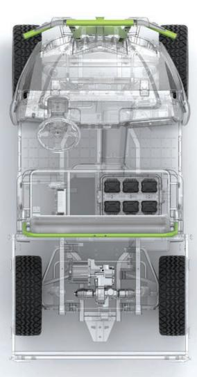
The GREENWORKS® commercial utility vehicle (UTV) is a dependable workhorse, equipped with a powerful 8kW max gTRON<sup>™</sup> drive system. This high performance UTV operates with the equivalent power of a 22hp / 352cc displacement petrol engine, its impressive 8kWh battery module provides up to 105km on a single charge for all day commercial use.
