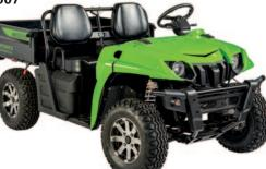
Voltage 82V Motor Type AC Induction Max Power Rating 15kW Main Gearcase Direct Drive Drive System Rear 2WD Front Diff Lock Electric Wheelbase 180cm Ground Clearance 216mm Brakes Hydraulic Disc Payload Capacity 454kg
