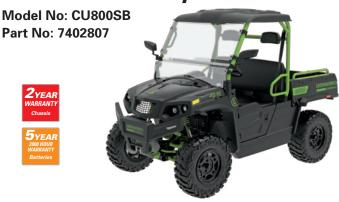
Voltage 82V Motor Type AC Induction Max Power Rating 15kW Main Gearcase Direct Drive Drive System 4WD Front Diff Lock Electric Wheelbase 184cm Ground Clearance 254mm Brakes Hydraulic Disc Payload Capacity 454kg Cargo Bed Capacity 250kg Tow Capacity 454kg Ground Speed Up to 43kph Runtime/Range Up to 120km Weight 795kg \* Available in Selected Stores only.
