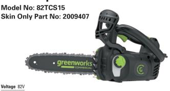
Motor Brushless Bar Length 10" (25cm) Chain Pitch 1/4" Chain Gauge .050" Chain Speed 24m/s Chain Tension With Tool Max Power 1.5kW
