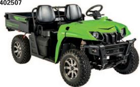
Voltage 82V Motor Type AC Induction Max Power Rating 15kW Main Gearcase Direct Drive Drive System Rear 2WD
